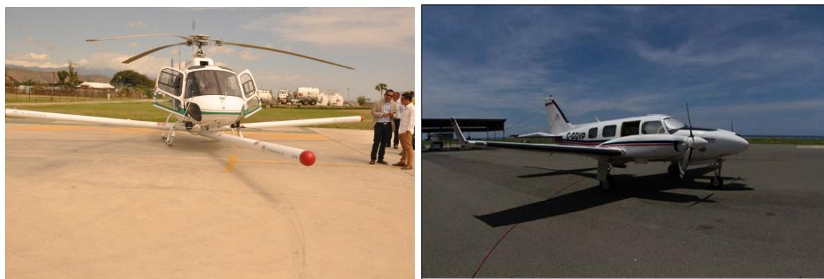
FIGURA 14: HELIKOPTRU BA PESKIZA MAGNETIKU-RADIOMETRIKU FIGURA 15: AVIAUN BA PESKIZA GRAVIDADE-MAGNETIKU
