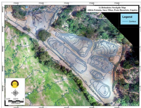
FIGURE 50: DRONE MAPPING AND STOCKPILE VOLUMETRIC SURVEY
